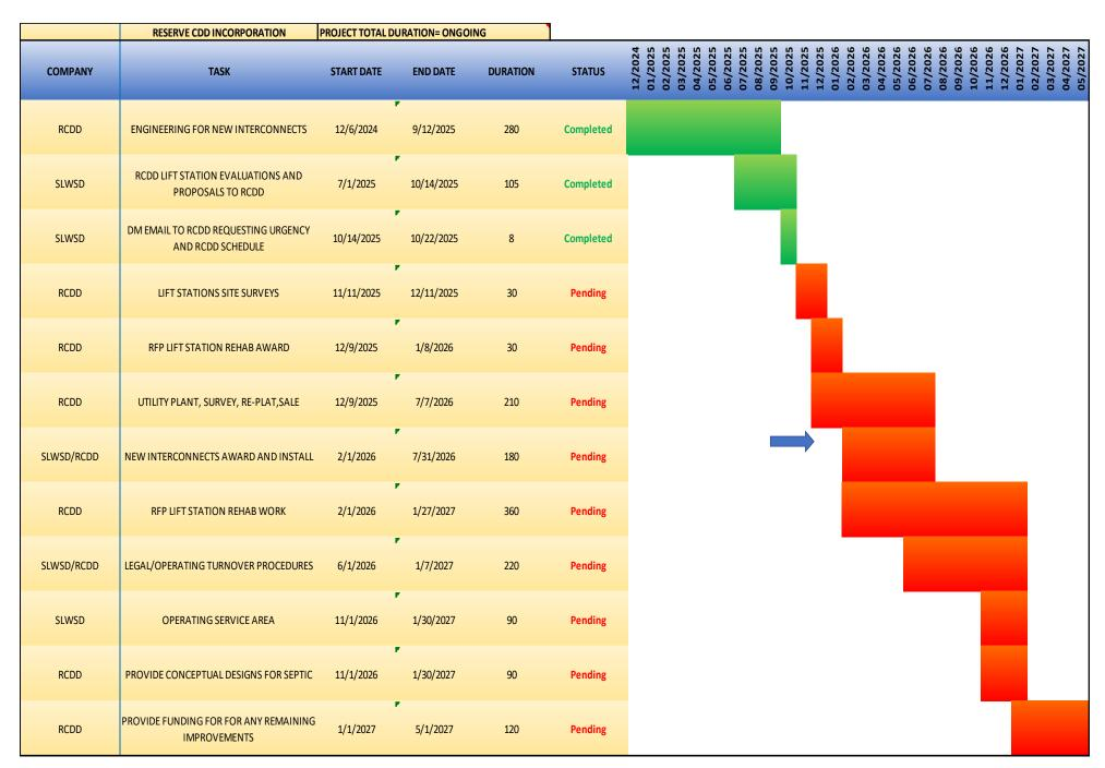
CRITICAL PATH: NEW INTERCONNECTS MUST BE INSTALLED AND TESTED
